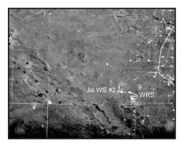
Figure 7. High-altitude aerial photo of area around WRS (11/97). Outlined area is a square one mile (1.62 km) on a side. Note small round dark areas west (left) side of photo along linear trends. Bachman (1973) attributed such features to caliche dissolution between paleodunes.
