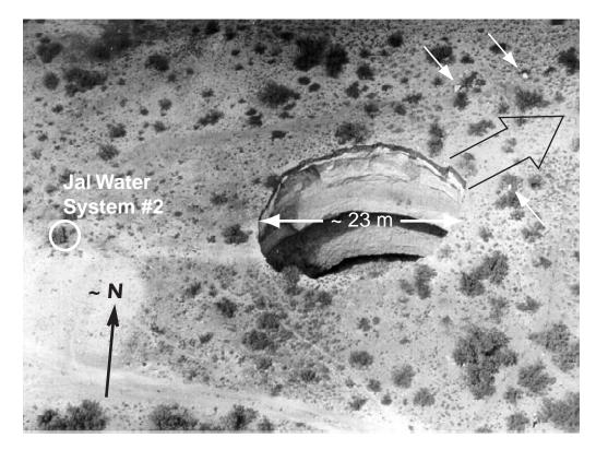
Figure 2. Lowangle aerial photo of WRS, taken to the north. Small arrows show the location of some larger clasts of Mescalero caliche blown northeast (outline arrow) by the collapsing material. The drillpipe for Jal Water System #2 is circled. Photo taken 9/ 15/98 by D.W. Powers.
